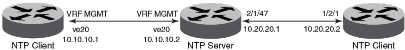
FIGURE 4 Use Case 2: NTP Server over Management VRF with One Client Using Management VRF and Another Client Using Ethernet
